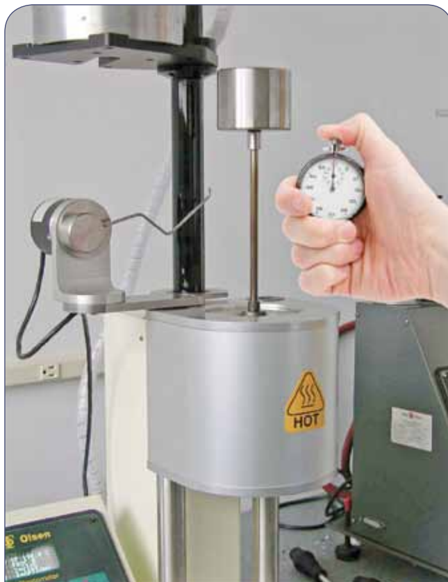
ASTM specifies 420 \pm 30 sec of preheat time for most materials.
