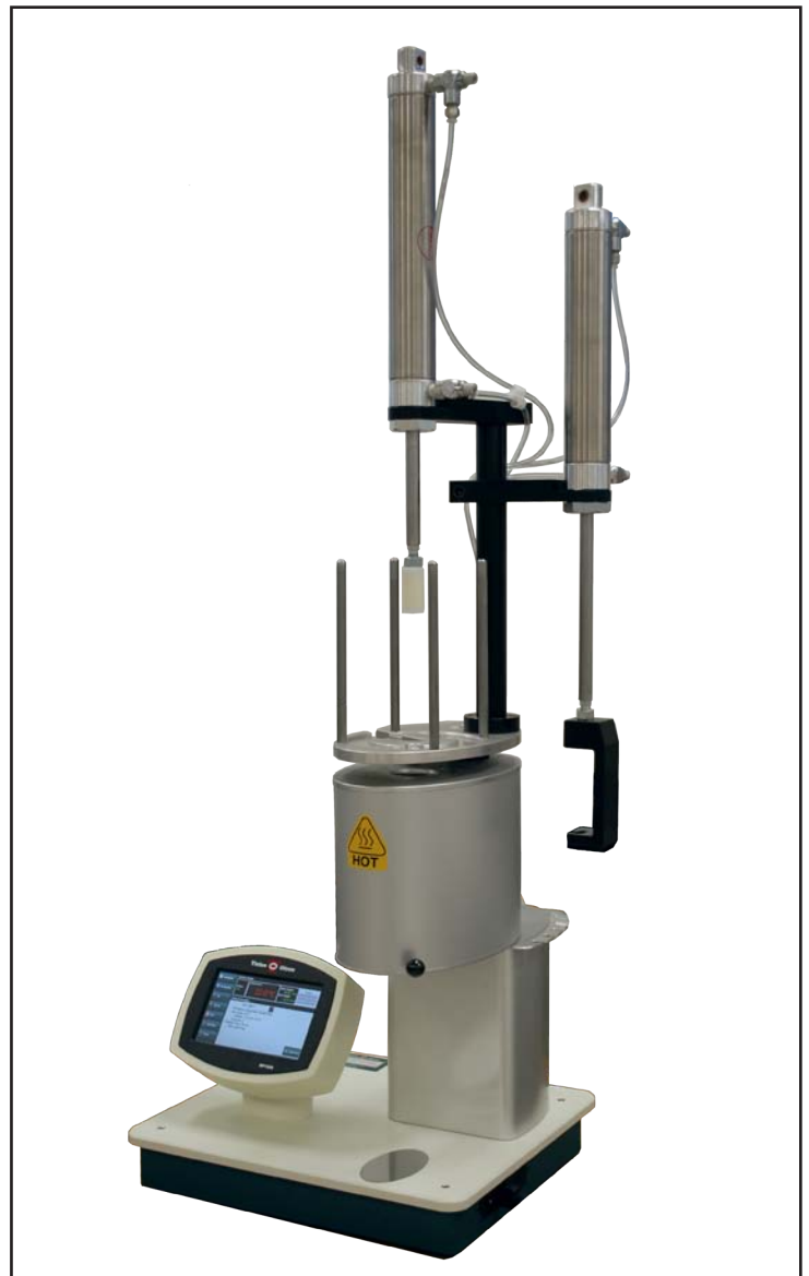
Fig 7. Model MP600 shown with lowered weight platform and pneumatic purge and pneumatic cleaning pistons for simplified rapid testing and cleaning.
